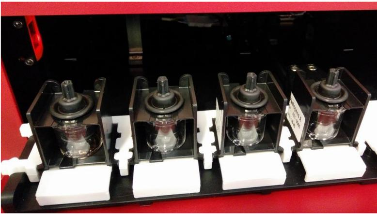
The barcodes of the hybcells in the rack have to face the inside of the device.
