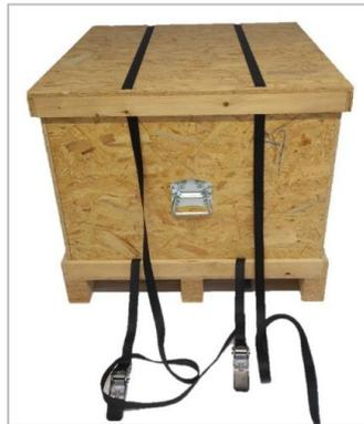
8. Attach the transport instructions on the top cover of the carrier box and tighten the lashing straps (using the attached ratchet spanners). If available, you can attach two shock indicators (No. 1, 'SHOCKWATCH') and tilt indicators (No. 2, 'TILTWATCH') each. Place the shock indicators on diagonally opposite corners. Place the tilt indicators on a long and a short side each.
