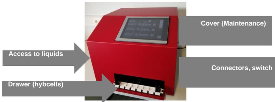
Connectors are located on the right of the device. They are used to connect the barcode reader or additional peripheral devices (e.g., keyboard, computer mouse, ethernet cable, etc.)
