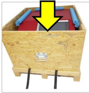
7. Thread the lashing straps into the provided holes of the top cover and put the top cover onto the carrier box. If there are no such holes provided, the straps are routed around the outside.
