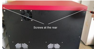
Remove two screws at the rear.
